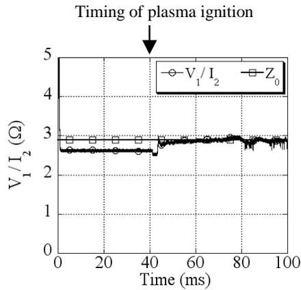
Fig.3 Evaluation of immittance circuit (Comparison of  $V_1/I_2$  with  $Z_0$ )
