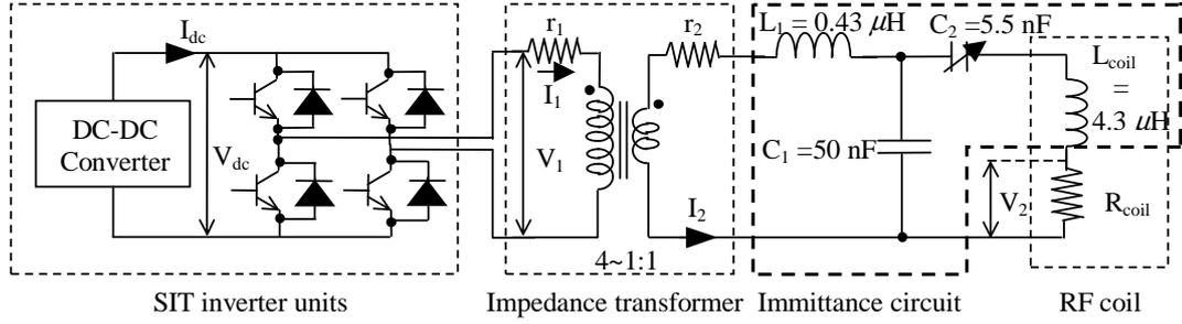
Fig.2 Equivalent circuit of the combined system (SIT inverter units, impedance transformer, immittance circuit and rf induction coil) for efficient rf inductive discharges)
