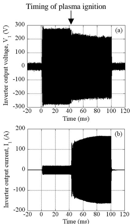
Fig.5 RF output voltage (a) and current (b) of the SIT inverter power source with immittance circuit
