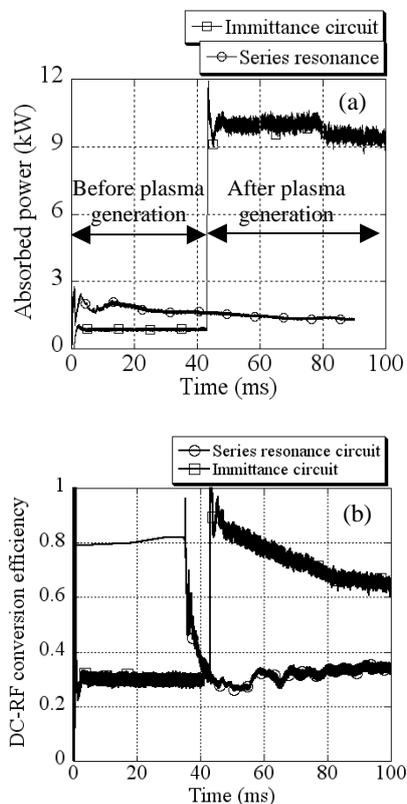
Fig.7 Comparison of absorbed rf power (a) and DC-RF power conversion efficiency (b) using immittance circuit with that of the series resonance circuit during plasma generation
