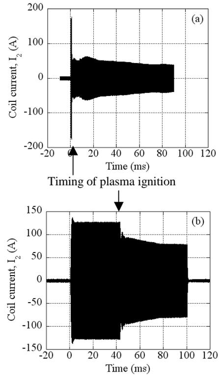
Fig.6 RF coil current waveform during plasma generation with series resonance circuit (a) and with immittance circuit (b)
