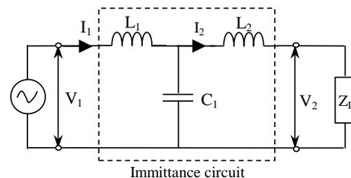
Fig. 1 T-LCL immittance circuit for constant current operation
