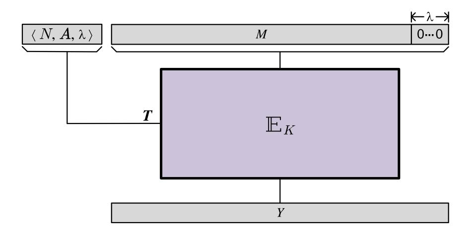
The natural construction, "enciphering-based AE," to make an RAE scheme from a generalized blockcipher
